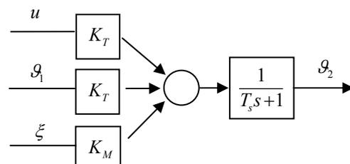
Fig. 2. Model of cooling by water injection
