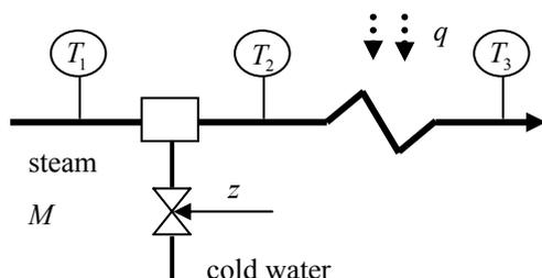
Fig. 1. Control of the temperature of overheated steam by cold water injection
