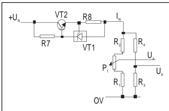
Fig. 1 The connection of power supply for bridge circuit.
