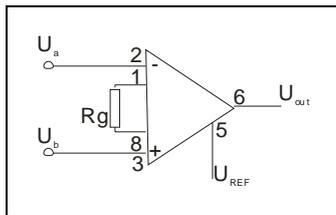
Fig. 4 Scheme of instrumentation amplifier
