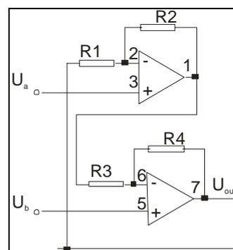
Fig. 3 Tested connection scheme of operational amplifiers with non inverting inputs
