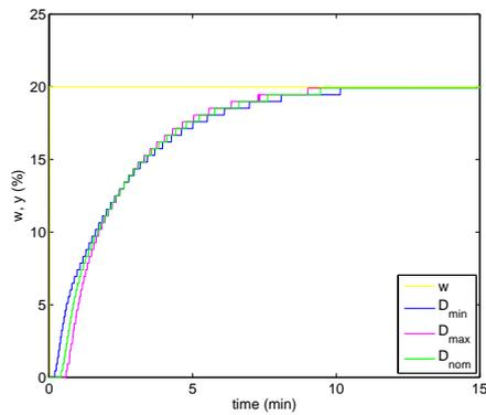
Fig. 8. Time responses for controller  $C_2$
