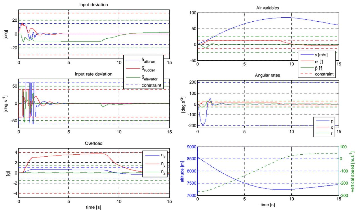
Figure 2 flight magnitudes during recovery
