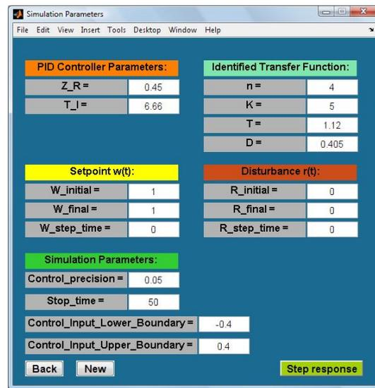
Fig. 8. Designed PI controller and simulation parameters
