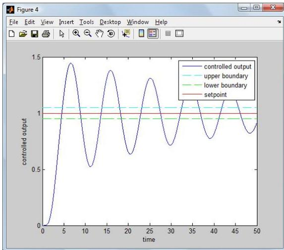
Fig. 9. Closed-loop step response generated by the software
