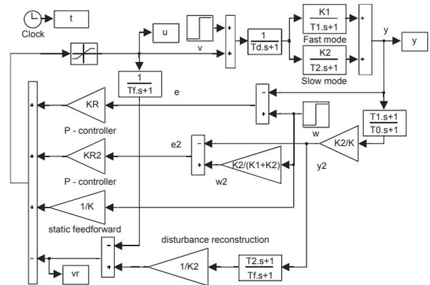
Fig. 2. Simulink model of the control loop with the P-PI controller
