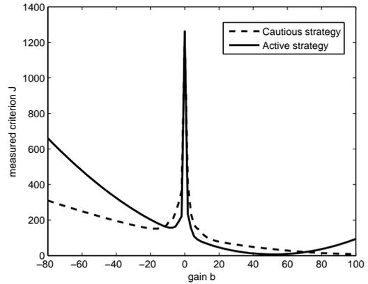
Fig. 4. Measured criterion values according to the real value of gain  $b$ , while  $\hat{b} = 10$  and  $\sigma_b^2 = 10^3$  is assumed.
