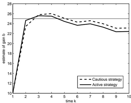
Fig. 3. The estimate of the system gain for  $b = 25$ , while  $\hat{b} = 10$  and  $\sigma_b^2 = 10^3$  is assumed.
