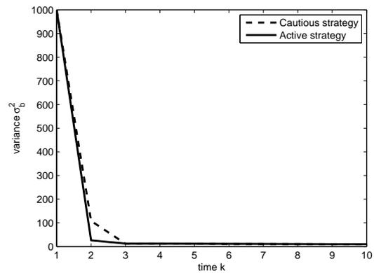
Fig. 6. The variance  $\sigma_b^2$  of the estimate of the gain  $b$  with  $b = 25$ , while  $\hat{b} = 10$  and  $\sigma_b^2 = 10^3$  is assumed.
