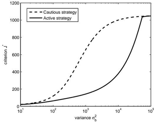
Fig. 1. The dependence of the optimal criterion value  $J^*$  on the parameter variance  $\sigma_b^2$  for cautious and active control strategy.
