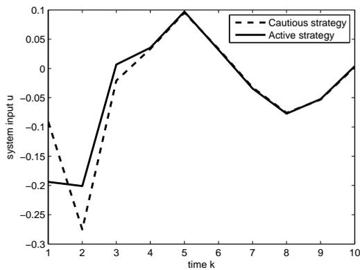
Fig. 2. Input to a controlled process with  $b = 25$ , while  $\hat{b} = 10$  and  $\sigma_b^2 = 10^3$  is assumed.
