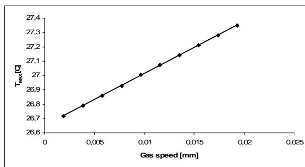
Fig.7. The dependence of  $T_{MAX}$  in semiconductor film on flow velocity  $v$ , gas–air, the diameter of the fluid channel  $d = 1,2 \text{ mm}$
