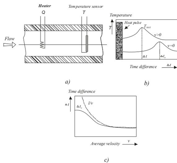
Fig. 1. Principles of the Time – of – flight sensor
