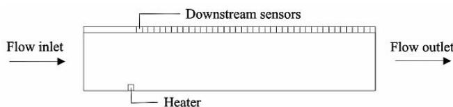
Fig.10. Experimental set-up of modified flow sensor
