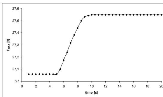
Fig.9. The time response of flow sensor: flow variation from  $30 \text{ ml/hr}$  to  $100 \text{ ml/hr}$ , the diameter of the fluid channel  $d = 0,8 \text{ mm}$
