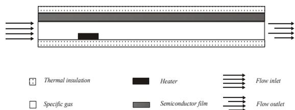
Fig. 2. Modified version of the time – of – Flight sensor
