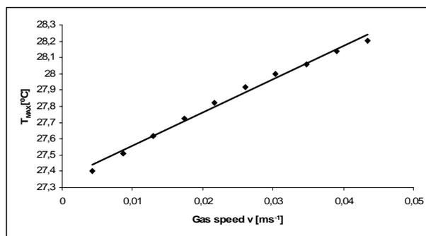
Fig.8. The dependence of  $T_{MAX}$  in semiconductor film on flow velocity  $v$ , gas – carbon dioxide, the diameter of the fluid channel  $d = 0,8 \text{ mm}$
