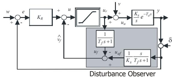
Fig. 1 DOB based PI<sub>1</sub> controller
