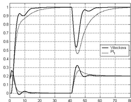
Fig.3 Transient responses of the PI controller tuned at the point (20) and the PI<sub>1</sub> controller responses with tuning (22) for the actual plant parameters (21)
