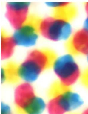
Fig. 1 Three-colour print sample with digital screening (scanned with zoom about 100)
