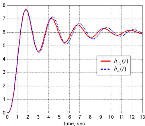
Fig. 2. Step-responses of object and identified model
