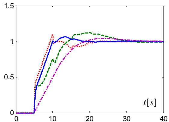
Fig. 8.  $F_2(s)$  reference tracking, step response. Settings: MO-PID (solid line), MO-PI (dash-dotted), Chien (dashed), Wang (dotted)
