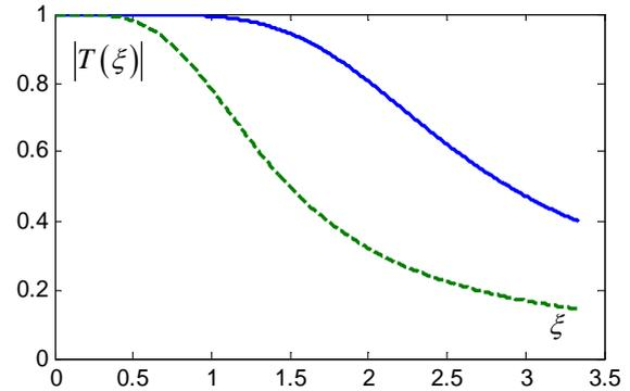
Fig. 4. Dependence  $\xi \rightarrow |T(\xi)|$  (solid line – PID controller, dashed line – PI controller)
