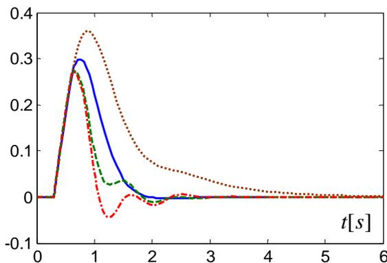
Fig. 9.  $F_1(s)$  load disturbance, step response. Settings: MO (solid line), Chien (dashed), Lopez (dash-dotted), Haalman (PI) (dotted)
