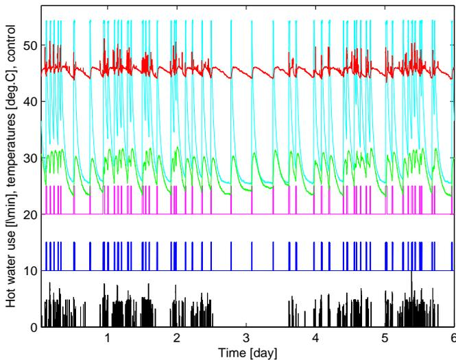
Fig. 4. Results of the predictive control algorithm performance.  $T_{wo}^3$  - red,  $T_{wo}^2$  - green,  $T_{zi}$  - cyan,  $F_w$  - black,  $Q_p$  - blue (scaled to 10-15),  $F_z$  - magenta (scaled to 20-25).
