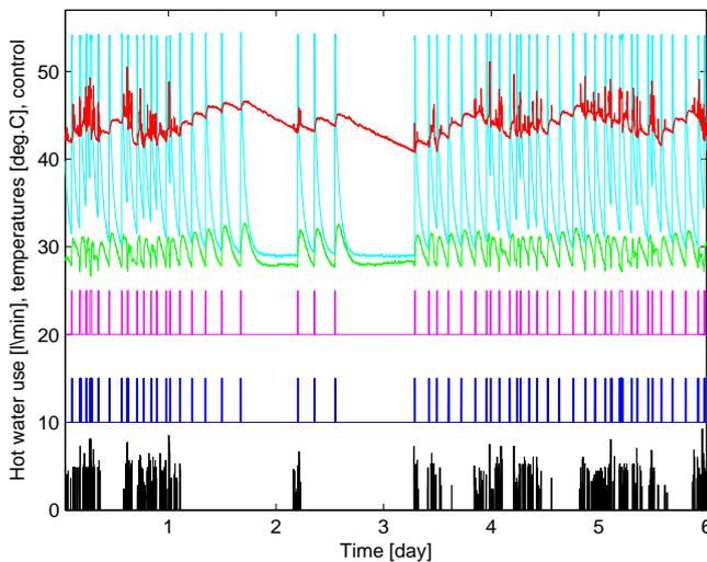
Fig. 2. Results of the standard on-off control performance.  $T_{wo}^3$  - red,  $T_{wo}^2$  - green,  $T_{zi}$  - cyan,  $F_w$  - black,  $Q_p$  - blue (scaled to 10-15),  $F_z$  - magenta (scaled to 20-25).
