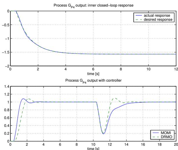
Fig. 7. Closed-loop responses of the process  $G_{p4}$  when using MOMI and DRMO method.
