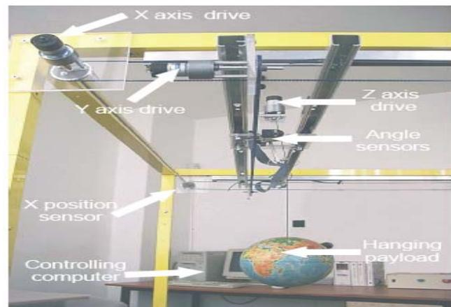
Fig.1. The 3DCrane setup
