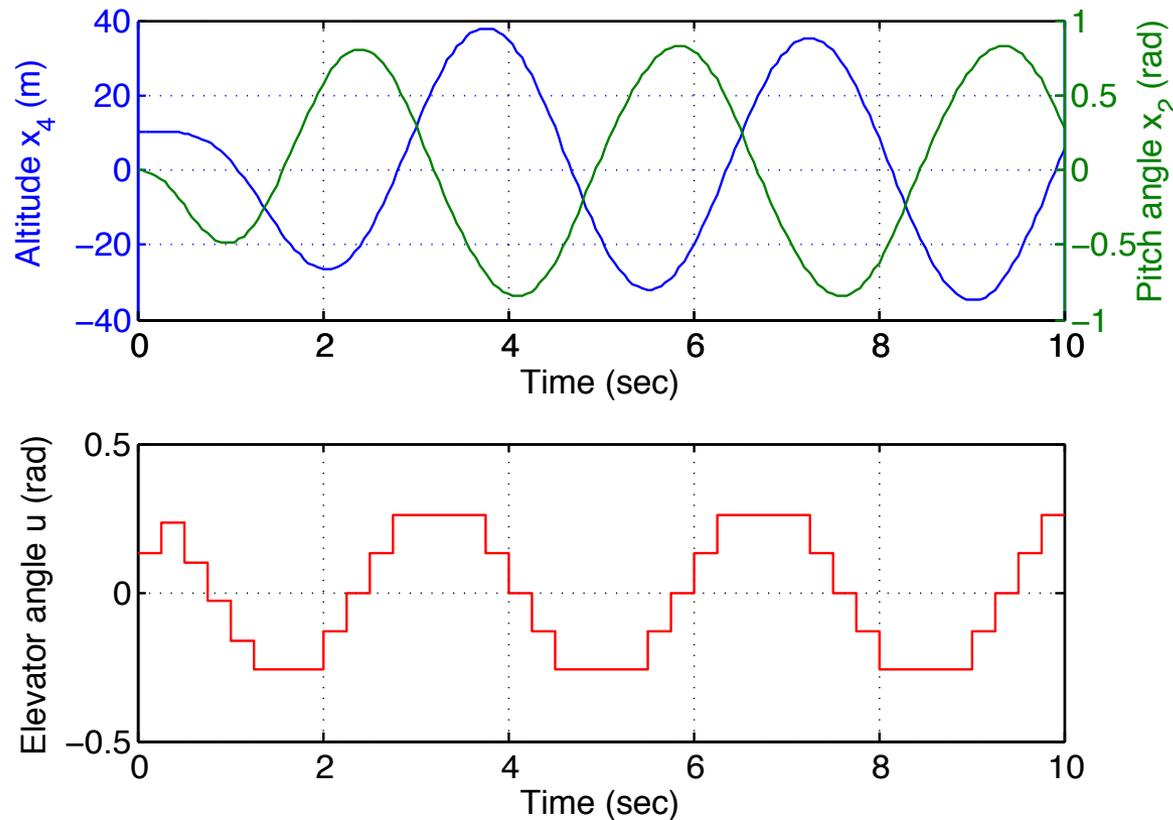
The MPC controller uses the knowledge that the elevator will saturate, but it does not consider the rate constraints.
