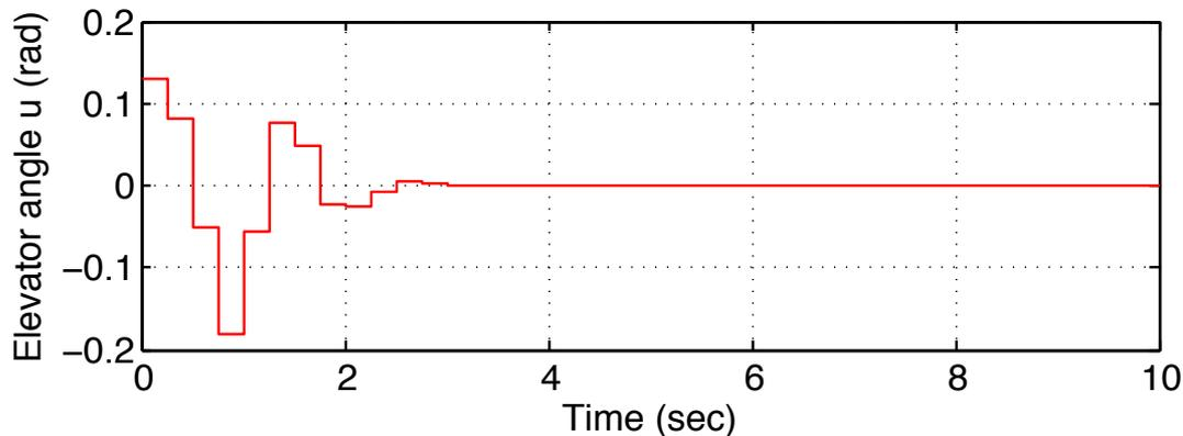
→ Inclusion of terminal cost and constraint provides stability
