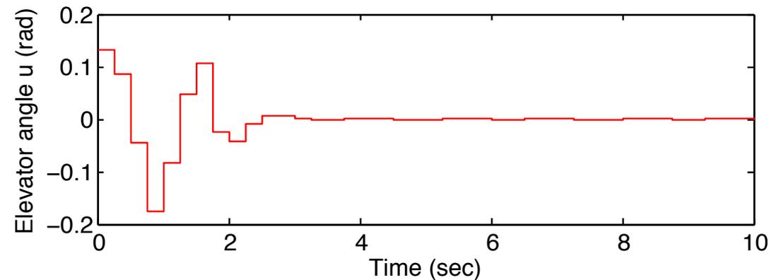
The MPC controller considers all constraints on the actuator
